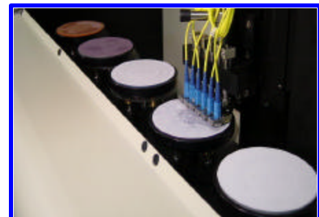
icon o 's multi-stage system processes connectors from air-polish through final UPC/APC finish.
