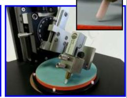
Bare fiber can be polished at variable angles using specialized workholders and adapters.=
