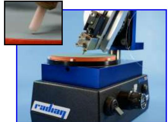
The patent-pending positioning feature, integrated in the common coupling mechanism, permits continual fiber advancement and retraction from the ferrule endface. This feature aids with fiber protrusion during polishing, attenuating transmitted power during system testing, and detector/transmitter proximity coupling control.
