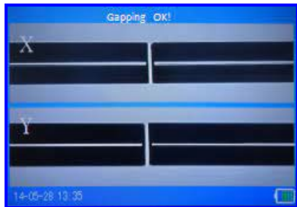
Prep fibers prior to fusion splicing for optimized alignment and low-loss joining.
