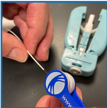
Clean containments and buffer residue during connector termination
